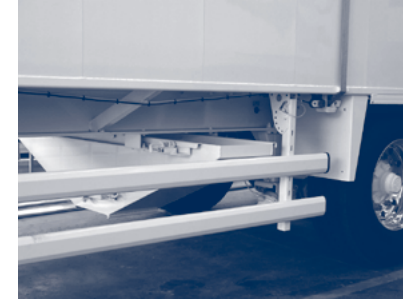
Figure 8.2.a. – Funnel behind side guard
