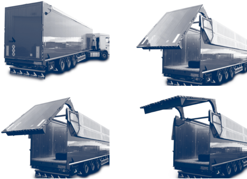
Figure 6.2.a. – Hydraulically operated top swinging door
