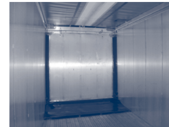
Figure 8.1.a. – Moving bulkhead with floor sheet
