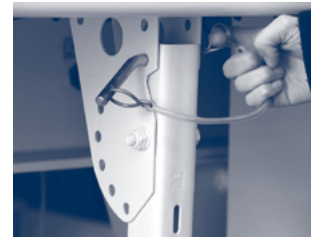
Figure 10.3.c. – Locking pin (left) and positioning pin (right)
