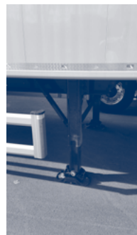
Fig 2.2.1.c. – Handle "steel type" landing leg
