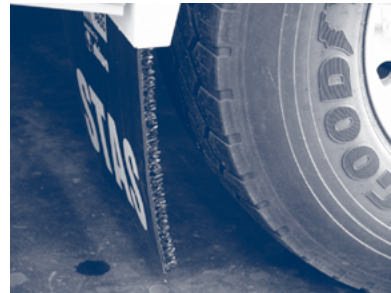
Figure 5.4.b. – Mud flap with spray suppression
