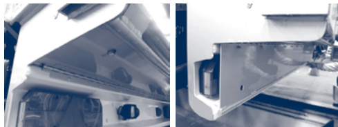
Fig 11.2.a. - Rear light protection up (left) and down (right)
