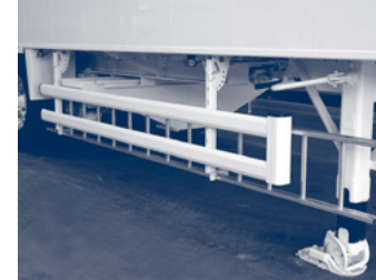
Figure 10.3.a. – Left hand side guard (right for "UK trailer")
