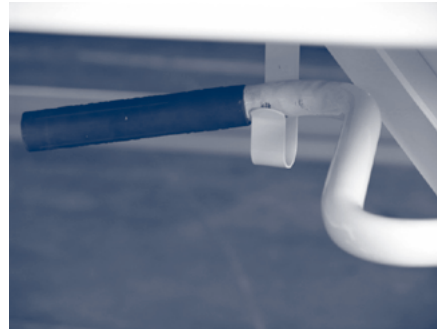
Fig 2.2.1.a. – Storage area for handle "steel type" landing leg
