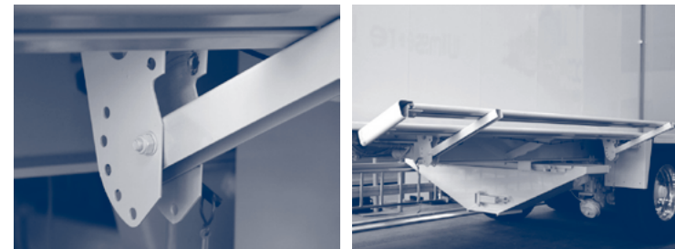
Figure 8.2.c. – Raised side guard
