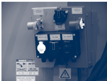
Figure 3.3.a. - Brake system connection
