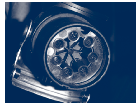
Figure 3.3.b. - 7-pin socket (left) and 5-pin socket (right)
