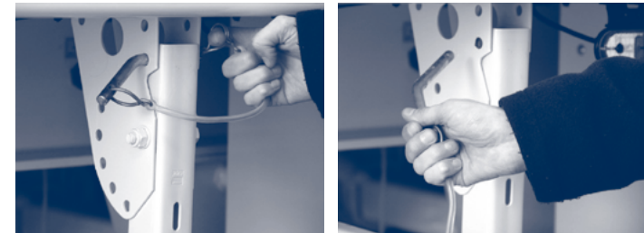
Figure 8.2.b. – Locking pin (left) and fixing rod (right)
