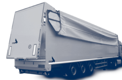
Figure 7.3.a. - Opened left hand section of roof net
