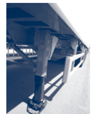
Fig 2.1.a. – Landing legs –aluminium type
