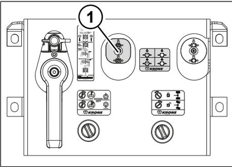
Fig. 5-21: Parking brake for central axle trailer
