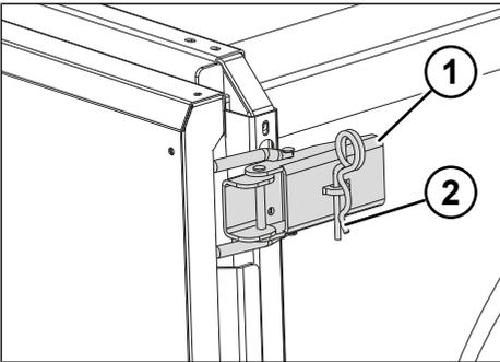
Fig. 5-41: Tension lock
