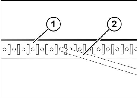
Fig. 8-5: Attach the telescopic lock rod
