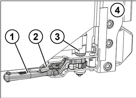
Fig. 6-23: Rear curtain tensioning device
