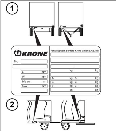
Fig. 1-1: Type plate attachment points
