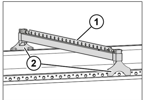
Fig. 8-11: Multi Block beam
