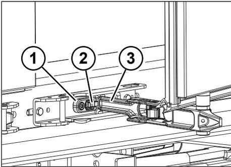
Fig. 6-10: Door lock lever engaged in the Door Fix
