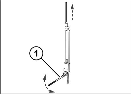
Fig. 6-51: Raising the lifting roof
