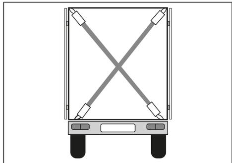
Fig. 7-4: Cross-bracing of the rear gantry
