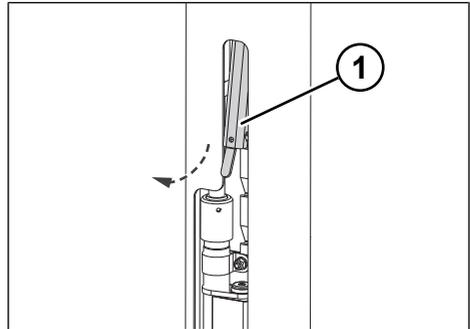
Fig. 6-53: Swivelling the adjustment bolt outwards
