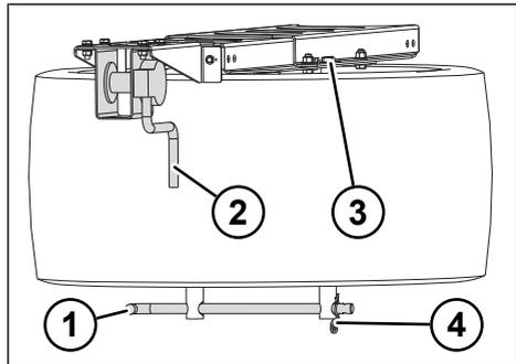
Fig. 5-37: Spare wheel with winch
