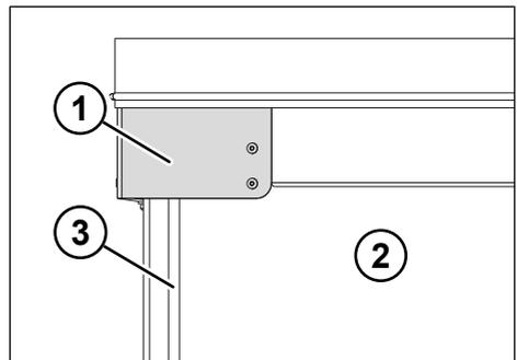
Fig. 6-22: Thread the channel rail
