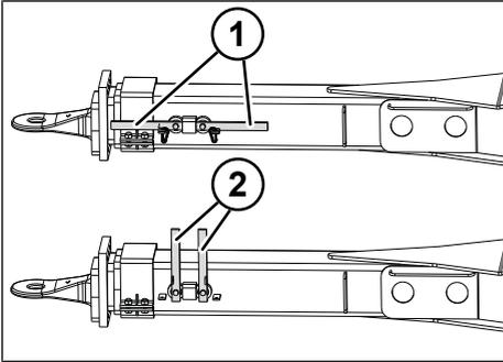
Fig. 5-12: Hand lever on the drawbar wale
