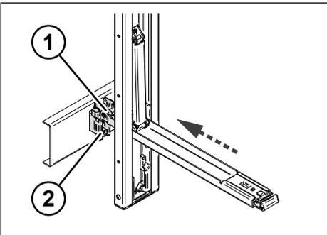
Fig. 6-36: Locking lever folded down
