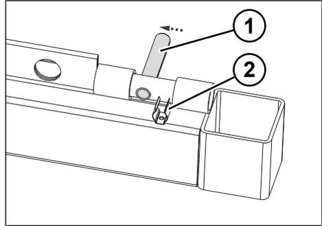
Fig. 8-13: Pulling out the locking lever
