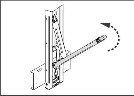
Fig. 6-35: Closing the locking lever
