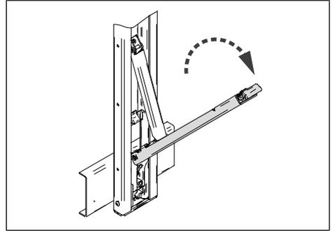
Fig. 6-33: Folding down the locking lever
