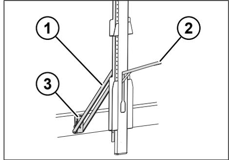
Fig. 6-30: Releasing the one-part fold-out post
