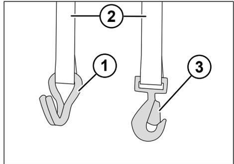
Fig. 8-1: Lashing material
