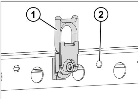
Fig. 8-7: Multi Lash with Multilock external frame
