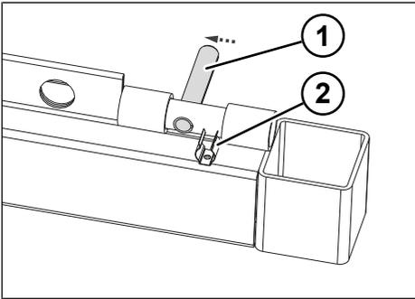
Fig. 8-16: Pulling out the locking lever
