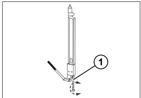
Fig. 6-50: Closing the drain valve
