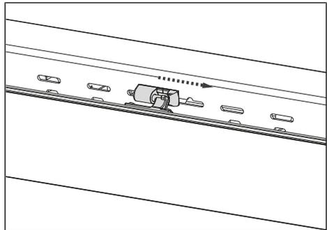
Fig. 6-27: Folding down the board wall
