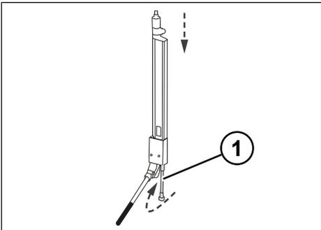
Fig. 6-52: Lowering the lifting roof
