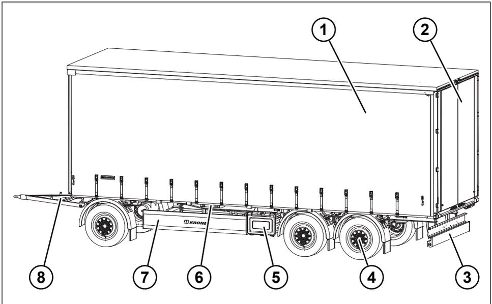
Fig. 3-3: Turnframe trailer (3-axle) with sliding curtain superstructure
