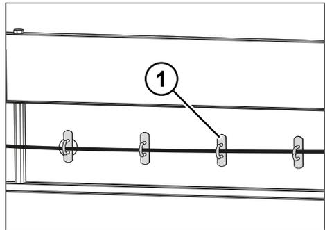
Fig. 6-43: Curtain cramps on the rear wall
