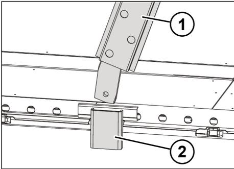
Fig. 6-40: Lifting out the tilting/plug-in post
