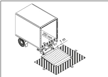
Fig. 6-13: Hazard area of the tail lift
