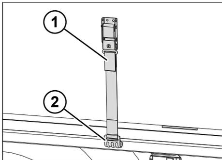
Fig. 6-15: Latch-type curtain buckle
