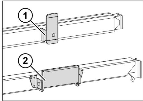
Fig. 8-19: Pallet retainer
