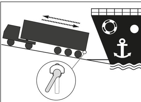
Fig. 7-5: Driving the trailer off the ferry
