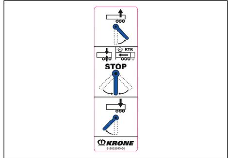
Fig. 5-19: Example pictogram of electronically controlled air suspension
