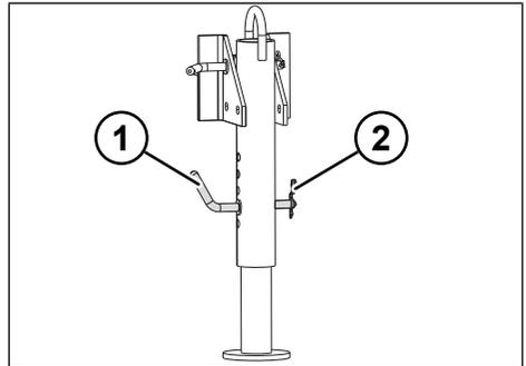
Fig. 5-10: Adjusting the height of the rear brace
