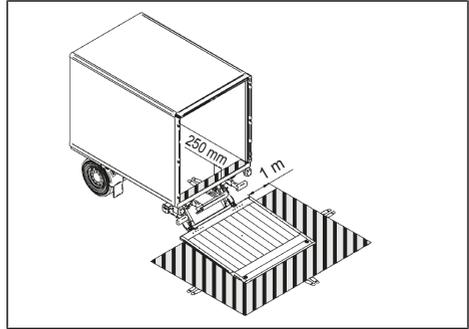
Fig. 6-11: Hazard area of the tail lift
