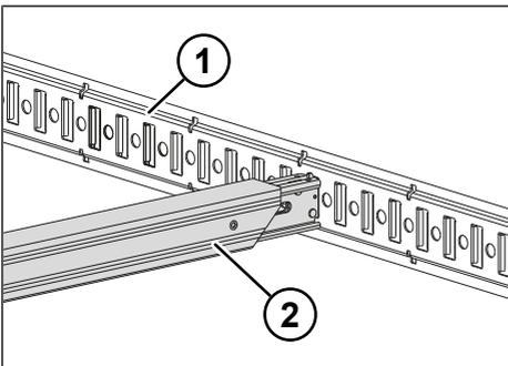
Fig. 8-6: Load securing rails with locking bars
