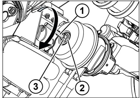
Fig. 5-16: Activating the emergency release screw
