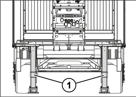
Fig. 5-2: Landing leg winches extended
