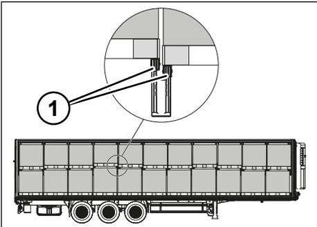
Fig. 8-17: Stepped arrangement of the support beams
