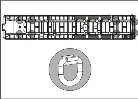
Fig. 7-4: Arrangement of the ferry rings
