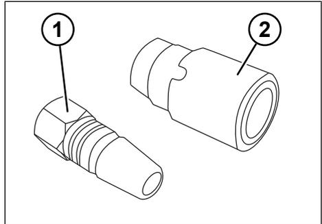
Fig. 5-13: C-coupling heads (trailer)
