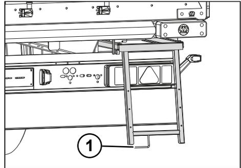
Fig. 5-23: Folding telescopic ladder in the function position
