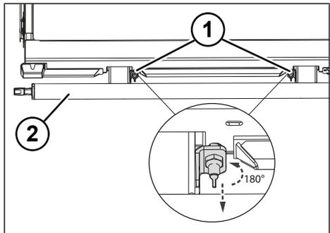
Fig. 5-26: Folding down the rear underrun protection
