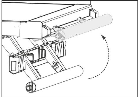
Fig. 5-25: Folding up the rear underrun protection
