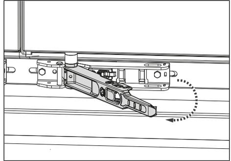
Fig. 6-3: Swivelling out the door lock lever
