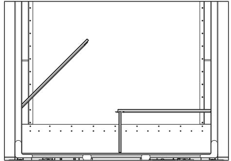
Fig. 6-25: Folding down the table without the landing leg foot
