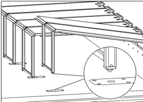
Fig. 6-24: Landing leg foot positioning aid
