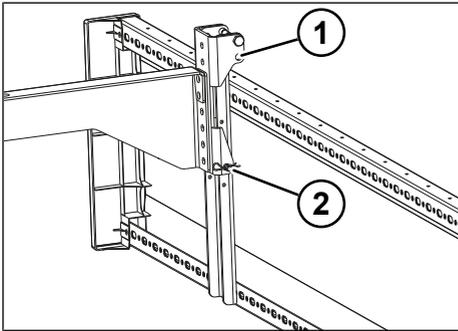
Fig. 5-30: Folded-down side collision protection ((rear view))
