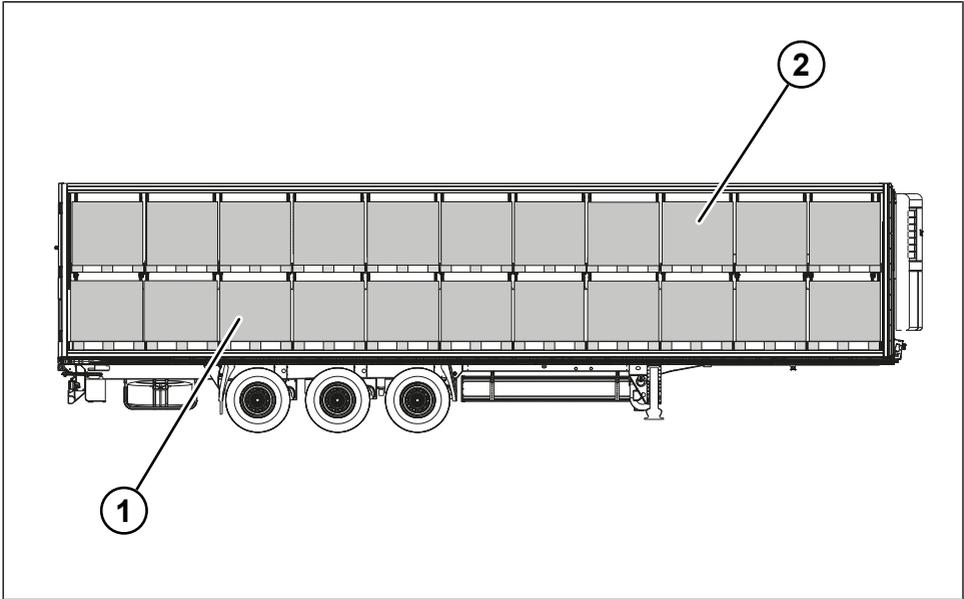
Fig. 8-16: Double-deck superstructure
