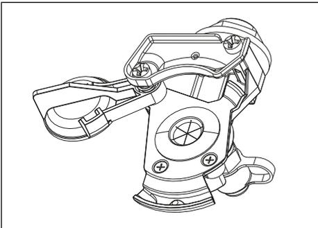
Fig. 5-11: Example of standard coupling head
