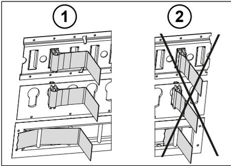
Fig. 8-1: Using tension straps
