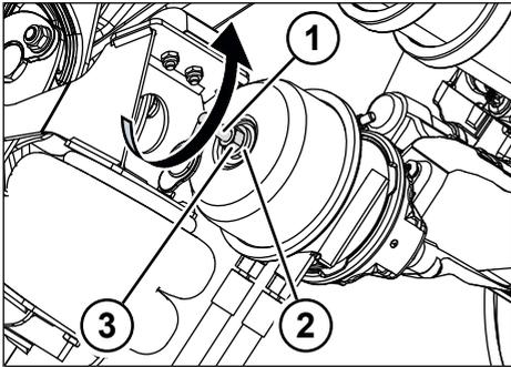
Fig. 5-17: Deactivating the emergency release screw
