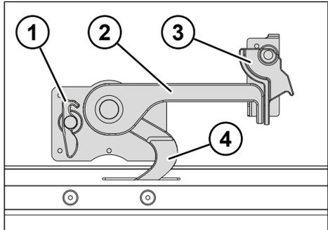
Fig. 6-14: Hook locking device
