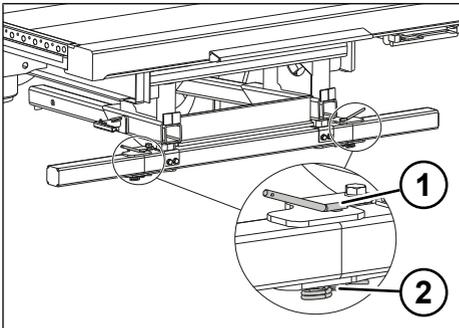
Fig. 5-27: Underrun protection that swivels out on both sides
