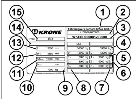
Fig. 1-1: Example type plate
