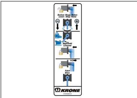
Fig. 5-18: Example pictogram of mechanically controlled air suspension
