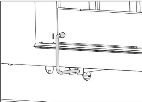
Fig. 6-7: Door leaf locked with the door stop
