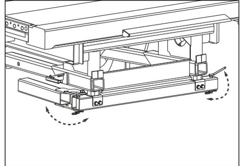
Fig. 5-28: Rear underrun protection swivelled in
