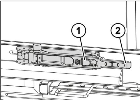
Fig. 6-2: Door lock with one-handed operation
