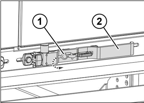
Fig. 6-4: Door lock with two-handed operation
