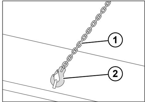
Fig. 8-3: Lashing chain with load hook
