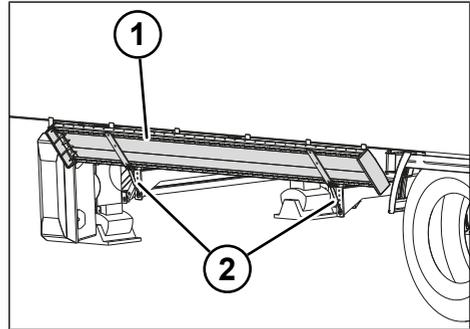
Fig. 5-29: Side collision protection folded up
