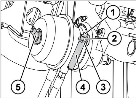
Fig. 5-15: Spring storage with emergency release device
