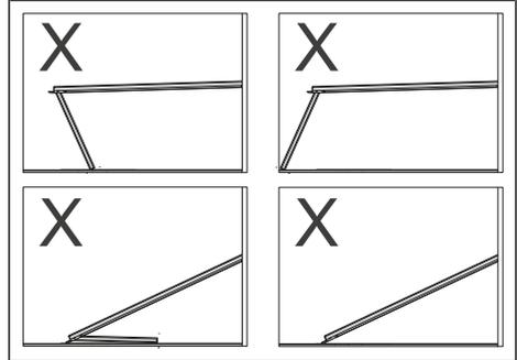
Fig. 6-21: Incorrectly positioned landing leg foot
