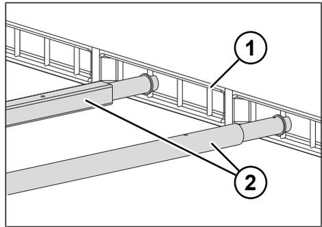
Fig. 8-9: Locking rods rod lashing rail
