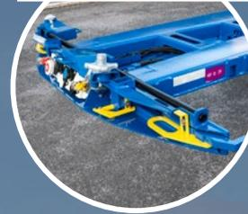
Rear lights installed in a protected location
